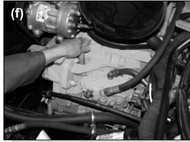
Inspecting the coolant hoses.
