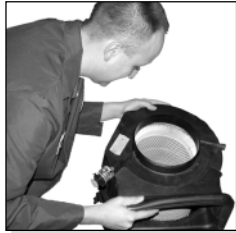
Inspect the engine air cleaner.
