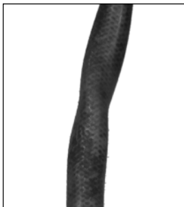
Partly collapsed inlet line shown.
